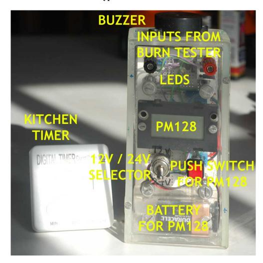
Piezo Buzzer (Note that this gets the full battery voltage across it, so must be 24V+ rated)
